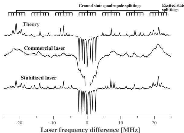
**Fig. 9.** Holeburning spectrum of  $\text{Pr:YAlO}_3$ .
