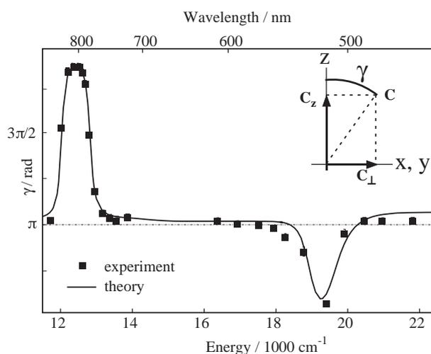
**Fig. 16.** Variation of the orientational angle  $\gamma$  with the laser wavelength. Filled squares represent experimental data, the solid line the theory. The inset shows the definition of the orientational angle  $\gamma$  in the molecular coordinate system.
