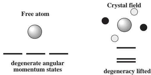
**Fig. 2.** Quenching of angular momentum by interaction with the crystal field.
