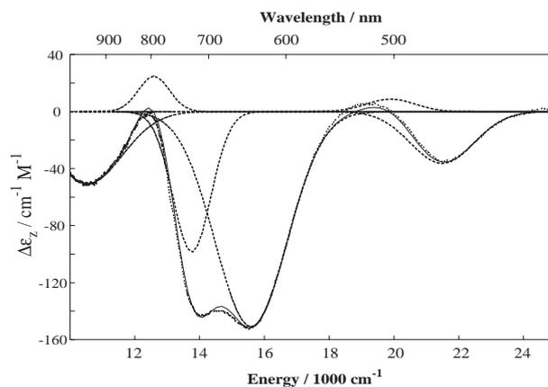
**Fig. 17.** MCD spectrum of Azurin (solid line) and its decomposition in six Gaussian bands (dotted lines).
