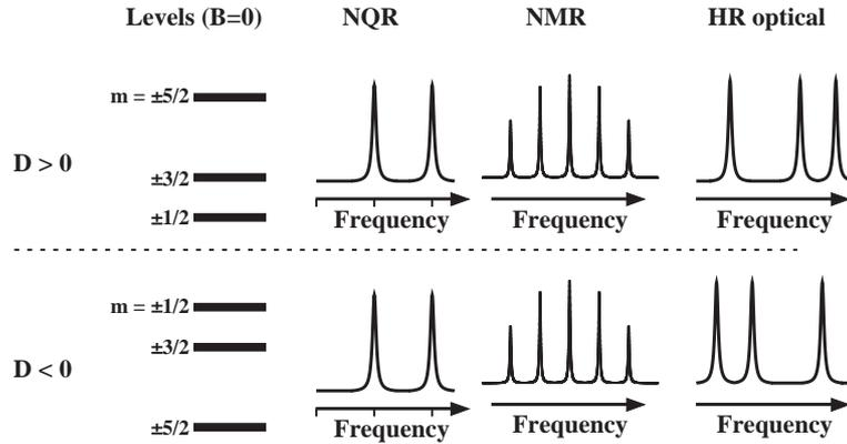
**Fig. 11.** Measurement of the nuclear quadrupole coupling by NQR, NMR and optical spectroscopy. Only the optical spectra distinguish the sign of the interaction.
