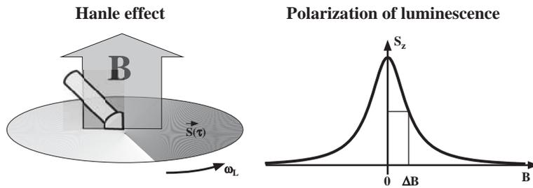
**Fig. 4.** Hanle effect: A magnetic field perpendicular to a circularly polarized excitation laser forces Larmor precession of the electron spins. The spin polarization of the excited electrons decreases therefore with increasing magnetic field strength.
