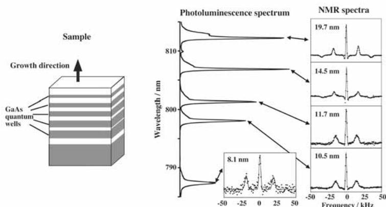
**Fig. 12.** Variation of quadrupole splittings in a multiple quantum well sample.
