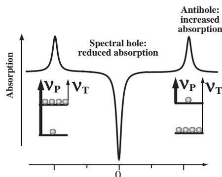
**Fig. 7.** Schematic representation of a holeburning spectrum. The hole represents reduced absorption, the “antihole” increased absorption. The separation between hole and antihole is equal to the transition frequency of the two spin states.
