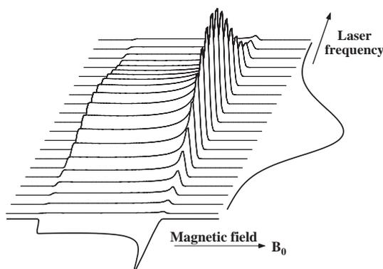
**Fig. 6.** Two-dimensional optically detected EPR (ODEPR) spectrum as a function of the laser frequency and the magnetic field strength. The result is a complete microwave resonance spectrum for each laser wavelength. The projections on the axes represent the conventional EPR and absorption spectra.
