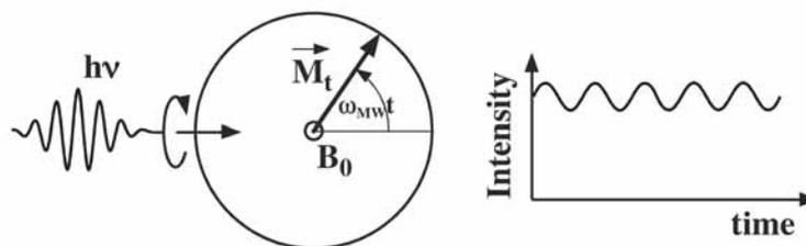
**Fig. 13.** Continuous wave excitation of EPR creates transverse magnetization  $M_t$  that rotates at the angular frequency  $\omega_{MW}$  around the static magnetic field  $B_0$ . The absorption of circularly polarized light is therefore modulated sinusoidally.
