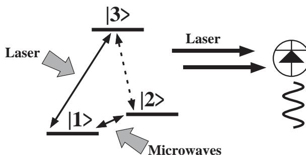
**Fig. 5.** Coherent Raman scattering from a three-level system. Laser excitation creates a coherence between levels  $|1\rangle$  and  $|3\rangle$  and microwaves between  $|1\rangle$  and  $|2\rangle$ . The resulting non-linear polarisation in the third transition creates a Raman wave.
