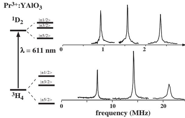
**Fig. 10.** Raman-heterodyne detected NQR spectra of Pr:YAlO<sub>3</sub>. All six resonances can be detected in a single wide frequency scan, but the low frequency part, which is associated with the NQR transitions in the electronically excited state has been expanded in the upper part of the figure.
