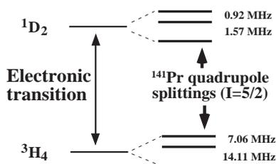
**Fig. 8.** Relevant level scheme for  $^{141}\text{Pr}$  doped into  $\text{YAlO}_3$ .
