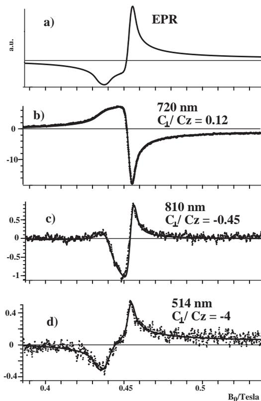
**Fig. 15.** a) Simulation of conventional EPR absorption (solid line) and dispersion (dashed line). b) to d) Dispersion type ODEPR spectra of azurin at different optical wavelengths in units of  $\Delta\epsilon \cdot 10^{-3} \text{ M}^{-1} \text{ cm}^{-1}$  (dashed line) and fit curves (solid line) [88].
